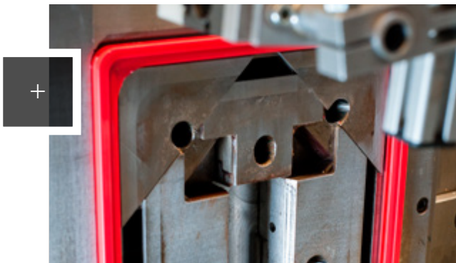
A glance in an opened injection mould with showcard frames and removal device
