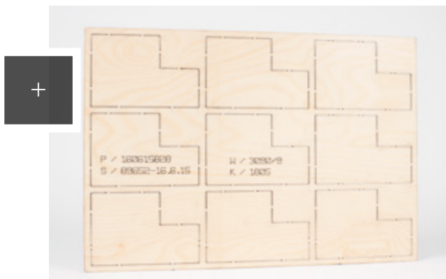
Punching tool with steel rule cutting technology for multiple cuts of shelf stoppers with side flags.
