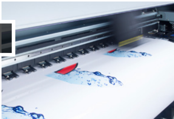
Digital printing on flexible materials such as for instance self-adhesive films up to a width of 1600 mm
