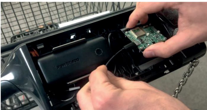
Illustration - Installing the receiver electronics in the handle
