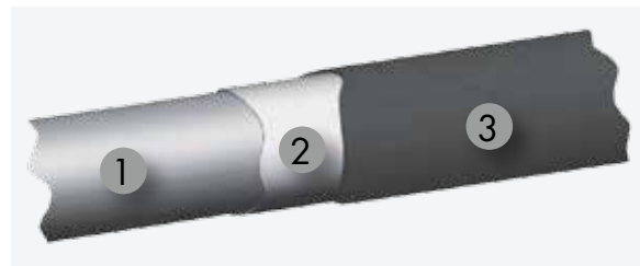
Innovative three layers: The surface coating protects the wire (1) against corrosion through galvanisation (2) and at the same time provides sound insulation thanks to a high-quality epoxy resin powder coating (3).
